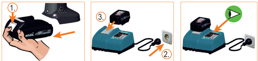
Fig. 5-1 Charging the battery
